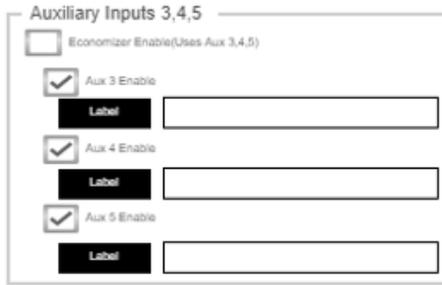
To use Aux 3,4,5 for Monitoring of Economizer temperatures, click the corresponding box in this section.
