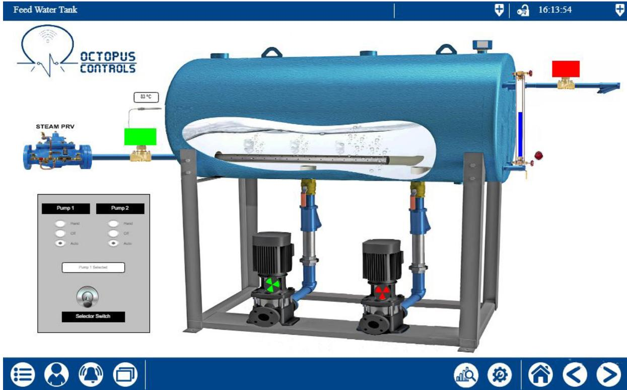
The FeedPump Operation can be changed on the control panel on this screen :
